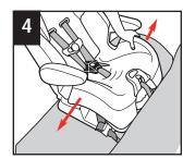
With weakest hand at belt path, tilt and push the child restraint forward and back, and from side to side. If the LATCH belts do not loosen, your child restraint should be secure.
